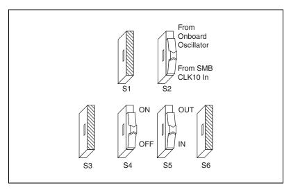
Figure C-3. Receive External CLK SMB and Drive to the Backplane Unterminated
